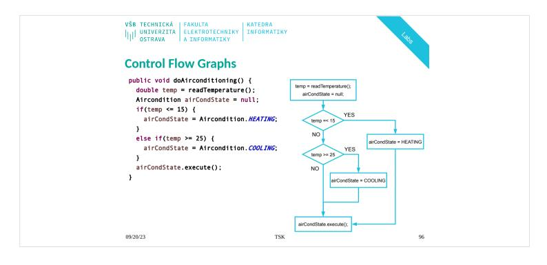
This is a small piece of code, which implements the temperature regulation. The function "adjust\_temperature" is called without arguments. The first thing it does is to read the current temperature, and then depending on the value, either the heater is switched on, the cooler is switched on, or the system is left untouched. The global variable *control* holds the current setting of the heater and cooler.
